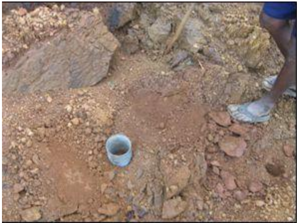
Photo 11: Collection of undisturbed sample just below the crown of Sasanwad slide no-3.
