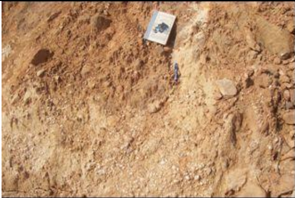
Photo 9: The weathered gneiss in the slide debris in the mid slope of Sasanwad slide no-3.
